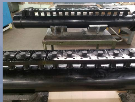
P-72 Manifold Header with CNC-machined Rectangular Flanges
