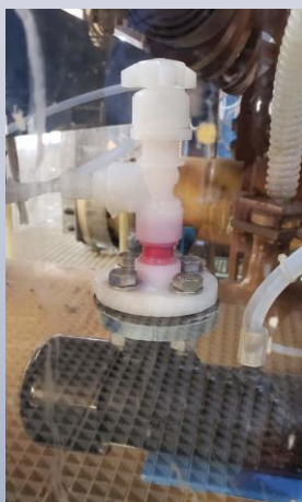
In-Service PVDF Flanged Vent Valve, with P-72 Header
