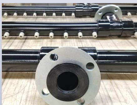
P-72 Base Flange Face with *Galvanized Steel Backing Ring
