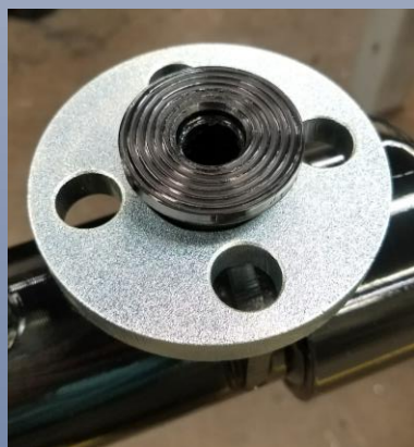
P-72 Vent Valve Flange Face with Galvanized Steel Backing Ring
