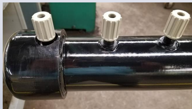
Solvent Socket Weld, Establishing Homogeneous P-72 Material
