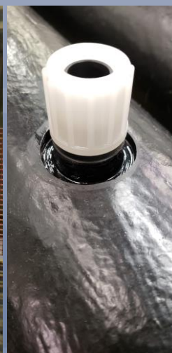
6" Double-Boss P-72 Header with FRP Overlay
