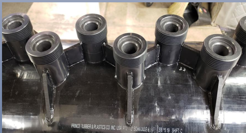
P-72 Manifold Header with CNC-machined Rectangular Flanges
