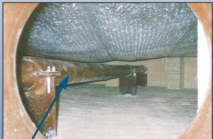
Typical hoop support shelf used when protuberances are present at the bottom of tank.
