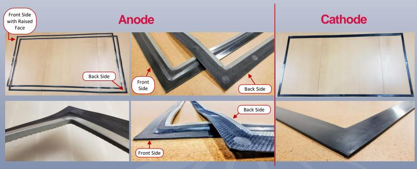
\* Anode Gaskets have: • Continuous Fluoroplastic Shield vulcanized on I.D. extending ~7mm up both sealing faces
