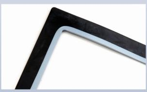
This SPECIAL compound 6962 EPDM exhibits resistance to most acids, bases and polar solvents such as water, phosphate ester, Ketones, alcohols, and glycols. EPDM swells considerably in aliphatic, aromatic, and chlorinated solvents. This compound is resistant to ozone attack and is weather resistant. We have found that 6962 generally outperforms any "commercial" grade EPDM.
